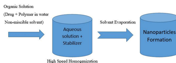
Figure 3. Solvent Evaporation Technique
